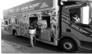
Latest 12-tonne 'Kerb-sort' design with variable-height, double-sided loading (no capacity for bulk bins)
