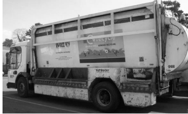
Current, discontinued 23-tonne 'Kerbsider' design with fixed-height, near-side loading and capacity for bulk bins
